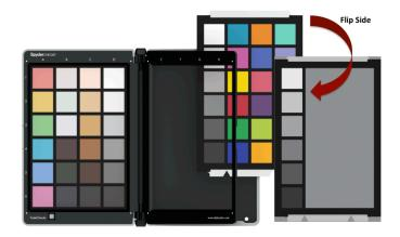
The SpyderCHECKR can be used for visual color comparisons, as well as with a number of third party software packages for camera profiling and other tasks. But most commonly, it is used with the SpyderCHECKR software in creating camera calibrations.
