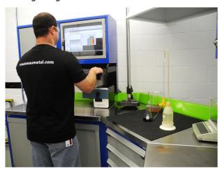
"We use Datacolor devices every day to approve each batch of paint we receive," Bernier says. "This allows us to ensure that the products will end up being perfectly matched." Rousseau previously used Konica Minolta solutions for color management, but switched to make this process easier. "We wanted to better document receipt of our paint and better follow the color deviations over time. Datacolor's software allows us to do exactly what we want in much less time than before."
